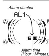
You can set five independent Daily Alarms. When an alarm is turned on, the alarm tone sounds when the alarm time is reached. One of the alarms is a snooze alarm, while the other four are one-time alarms. You can turn on an Hourly Time Signal that causes the watch to beep twice every hour on the hour.
