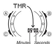
The countdown timer can be set within a range of one minute to 60 minutes. An alarm sounds when the countdown reaches zero. The countdown timer also has an auto-repeat feature and a progress beeper that signals the progress of the countdown.
