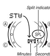
The stopwatch lets you measure elapsed time, split times, and two finishes.
