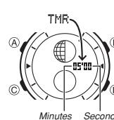
The countdown timer can be set within a range of one minute to 60 minutes. An alarm sounds when the countdown reaches zero. The countdown timer also has an auto-repeat feature and a progress beeper that signals the progress of the countdown.
