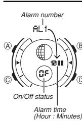
You can set five independent Daily Alarms. When an alarm is turned on, the alarm tone sounds when the alarm time is reached. One of the alarms is a snooze alarm, while the other four are one-time alarms.
