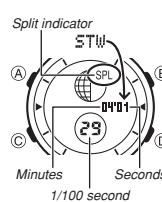
The stopwatch lets you measure elapsed time, split times, and two finishes.
